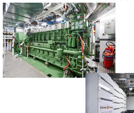
Main engines: Two ABC 8/6 DZC type engines 1.500/1.000kw
